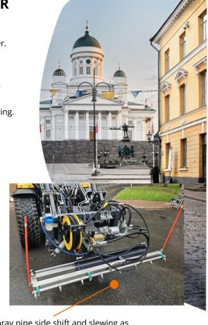
Spray pipe side shift and slewing as well as a manual pressure washer for reaching difficult spots as standard equipment.
